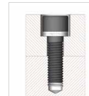
Countersunk socket head bolt secured in position
